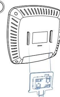
② Hook the stationary end of the mount bracket to the T-rail.
